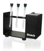
The ESR-Auto Plus automated analyzer is designed to accurately and precisely measure the sedimentation rate of erythrocytes in ESR-Vacuum Tubes.
